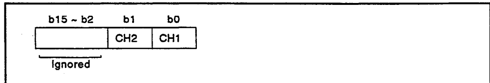
Fig. 3.7 Analog Output Enable/Disable Channel Area Data Map
